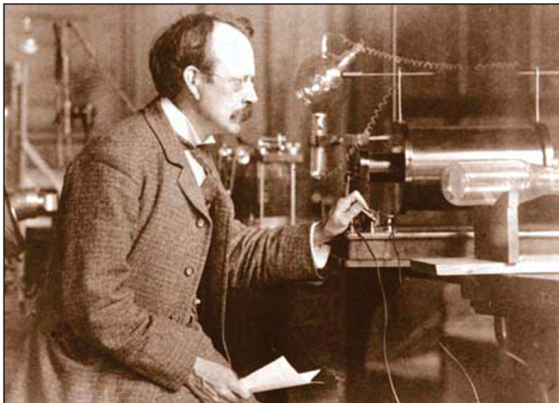
FIGURE 1: J. J. Thomson and a cathode ray tube used to perform some of the first m/z measurements. Deflection of the electron was observed once the electric field was turned on.
